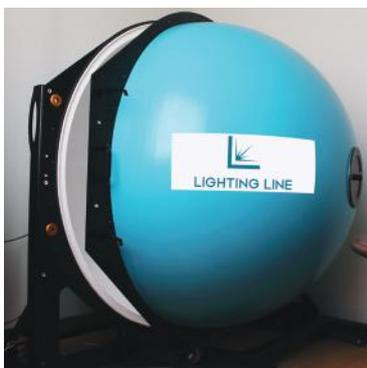
The second device we systematically rely on to test our products is our integrating sphere spectroradiometer, which makes us able to measure the spectral radiance of our strips and thus to draft ad hoc test reports providing information on their efficiency, color temperature, wavelength, light quality (CRI) and many other features.
